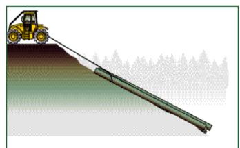
Figure 1 Tractor parked on level ground
